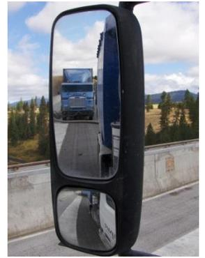
One way to reduce blind spots to the rear is to correctly adjust your mirrors. Many drivers adjust the side or 'wing' mirrors so that they see mostly what is behind them and much of the mirror view is taken up with view of the side of the vehicle. We don't need to see the side of the vehicle that we are driving. We need to see what's going on in the blind spots.
